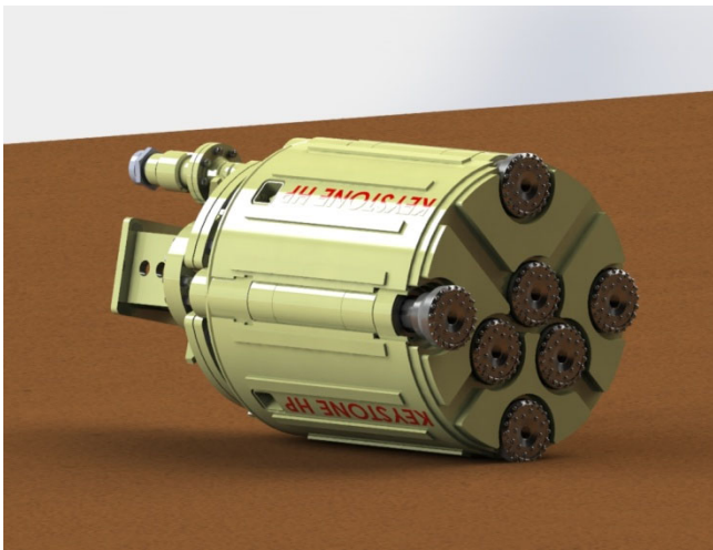
Figure 44: Bit Installation: Pass Chuck Splines
