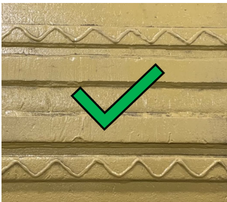
Figure 55 – Proper pattern on wear bars
