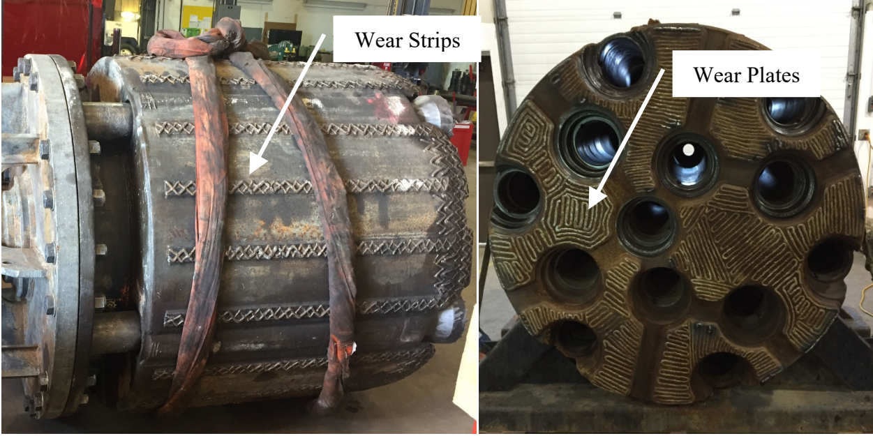
Figure 51: Hard Facing Example
